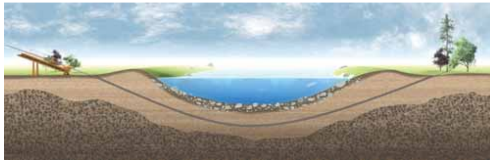
Horizontal directional drilling (HDD) uses a drilling rig on the surface to drill and install a pipe underground to avoid environmental disturbance.
