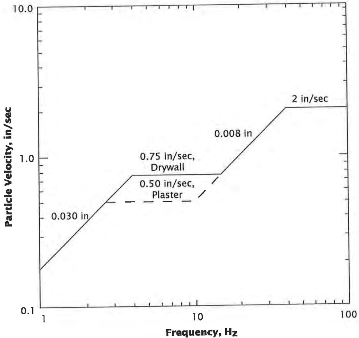
Vibration limits to prevent cosmetic damage in homes from blast-induced vibrations (U.S. Bureau of Mines, 1980). Note that the measured vibrations fall below the minimum 0.1 inch per second value on the horizontal axis.
